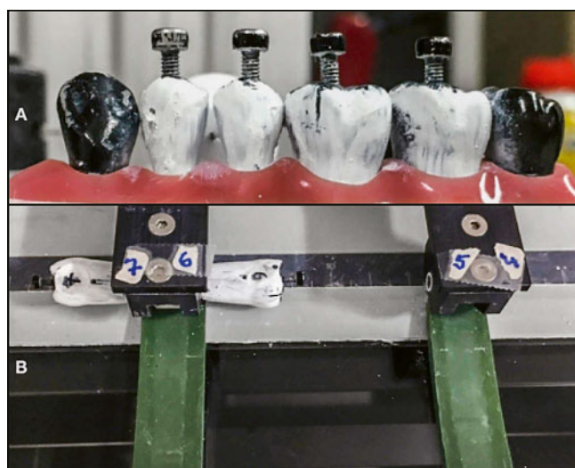
Fig. 3 A: Anatomical model consisting of black plastic teeth coated with a titanium dioxide/ethanol slurry. B: The teeth were removed and rolled over the scanner for evaluation.
